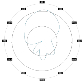
PA MMB0727-8X 2100Mhz, port 1, azimuth
