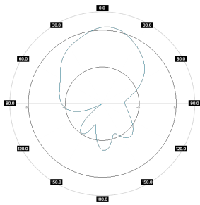
PA MMB0727-8X 2100Mhz, port 1, azimuth
